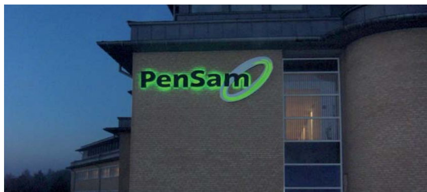
Aluminium logo and text with built-in LED lighting
